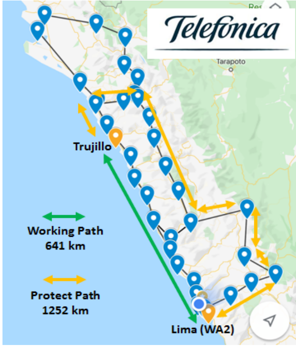
Fig. 1: Bi-directional transmission: working and protection fiber
