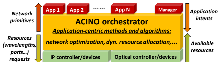
Fig. 1. ACINO SDN orchestrator architecture and communication with network applications and infrastructure.
