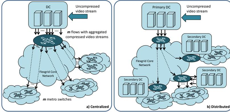
Fig. 1. Centralized (a) and distributed (b) architectures.
