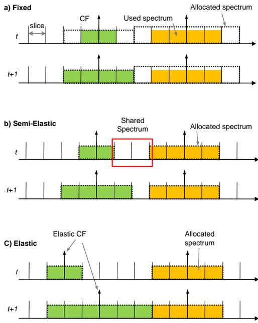
Fig. 2. Three spectrum allocation policies for time-varying traffic in a flexgrid network. Two time intervals are observed:  $t$  before and  $t+1$  after spectrum adaptation has been performed.
