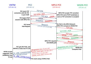
Fig. 2. Multi-PCE/VNTM signaling for coordinated multi-layer path computation. Note that in this example, the IP addresses of the PCC and the source node within the path computation request differ. As mentioned above, this is because the PCC could be an NMS. In the next section, we will examine this case in further detail.
